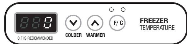
**NOTE:** °F/°C display control-press this control to change the displayed temperature to °F or °C.
